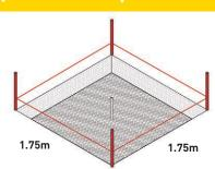
MARK & DIG To get started, mark out a 1750mm x 1750mm square base foundation on the site you want the fire pit located. The excavation is 100mm larger on each side of the completed planter.
